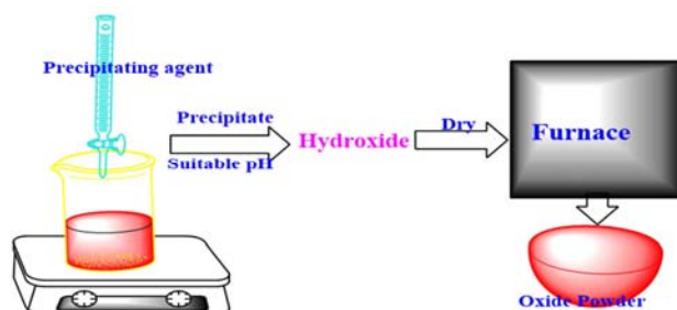
Figure 6. Synthesis of photonanocatalyst by co-precipitation method.
